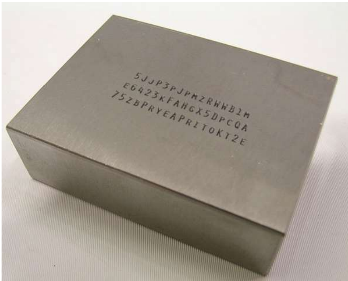
Figure 2.5: High durability Bitcoin key laser-engraved on a tungsten brick. Photomontage by deepceleron, original image from Avery Tools website, http://www.averytools.com/prodinfo.asp?number=6004 .
